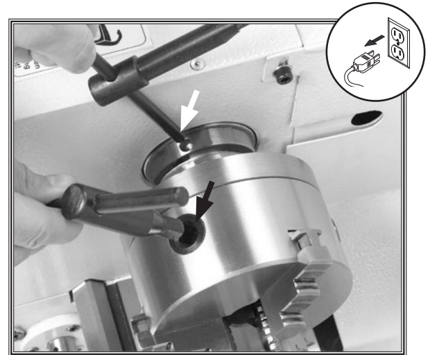
Figure 7. Inserting chuck keys to loosen or tighten the chuck onto the spindle.
